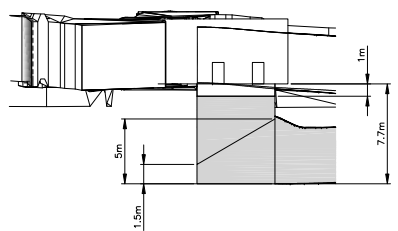
NORTH VIEW OF WATER CATCHMENT SUMP SCALE 1:200
