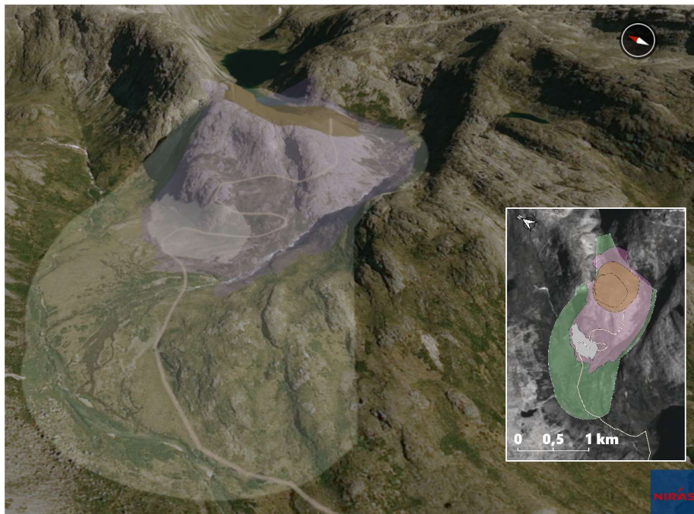
Figure 28: Visualization of mine- and blast site showing the gorge and ridge potentially acting to prevent dust dispersion of >30 \mu\text{m} particles to the south. Purple (top) marks expected active area with visible dust spread, light green (bottom) marking is expected inactive area, affected by light particle dispersion by wind.
