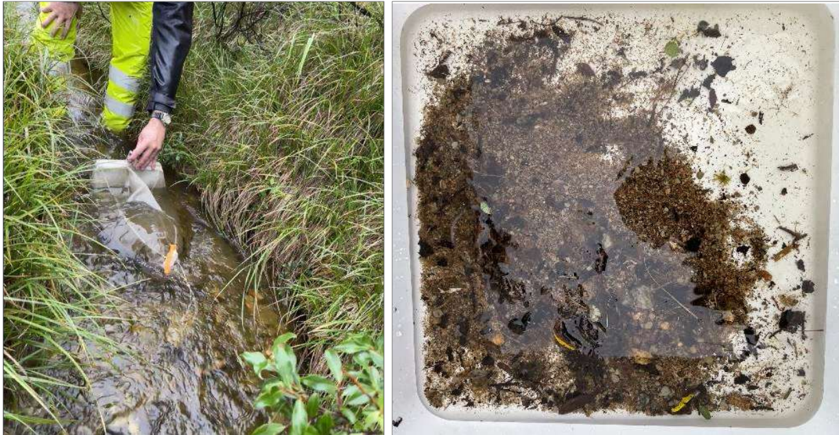
Figure 51: Kick sampling (left) and example of sample (right).
