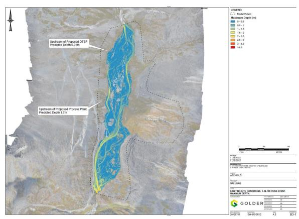
Figure 25: Maximum Flooding Depth 1-in-100 year event (from Golder, 2022e)
