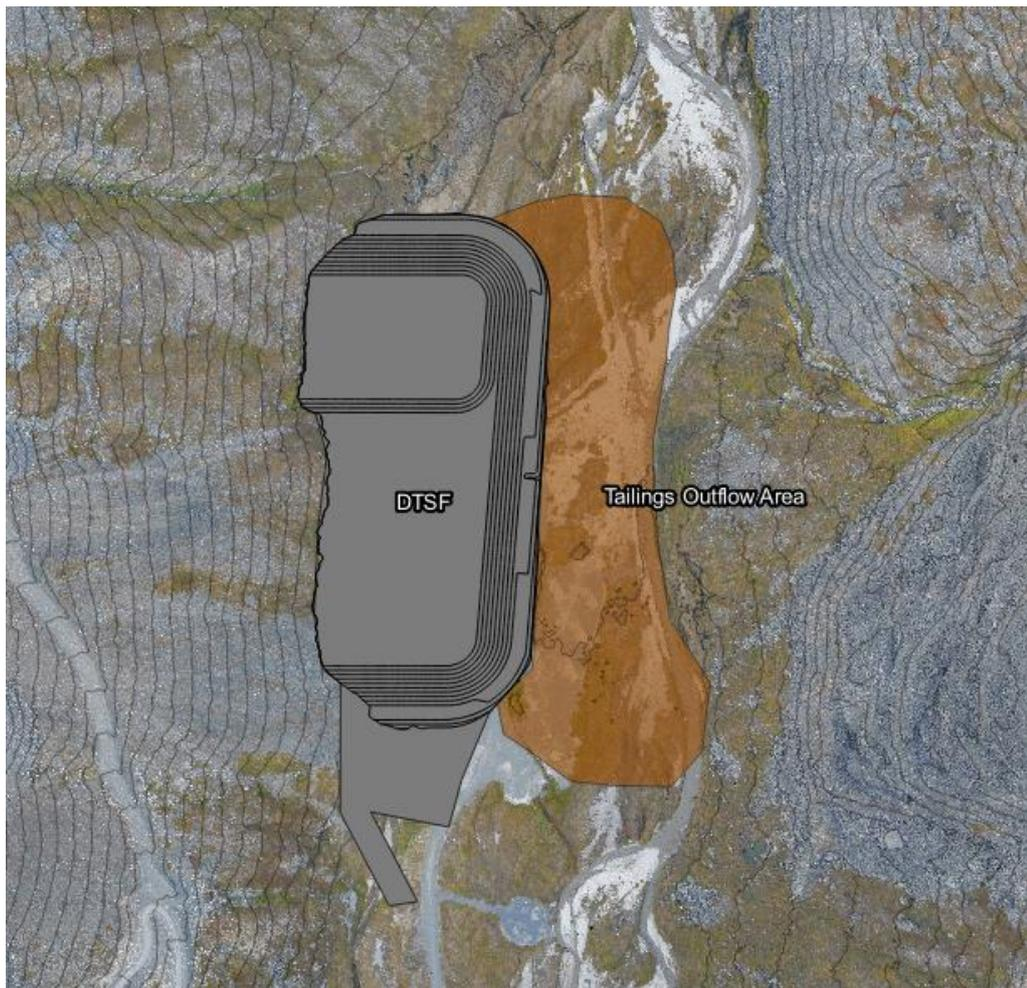
**Figure 38 : Projected tailings outflow area – Sunny day scenario**
