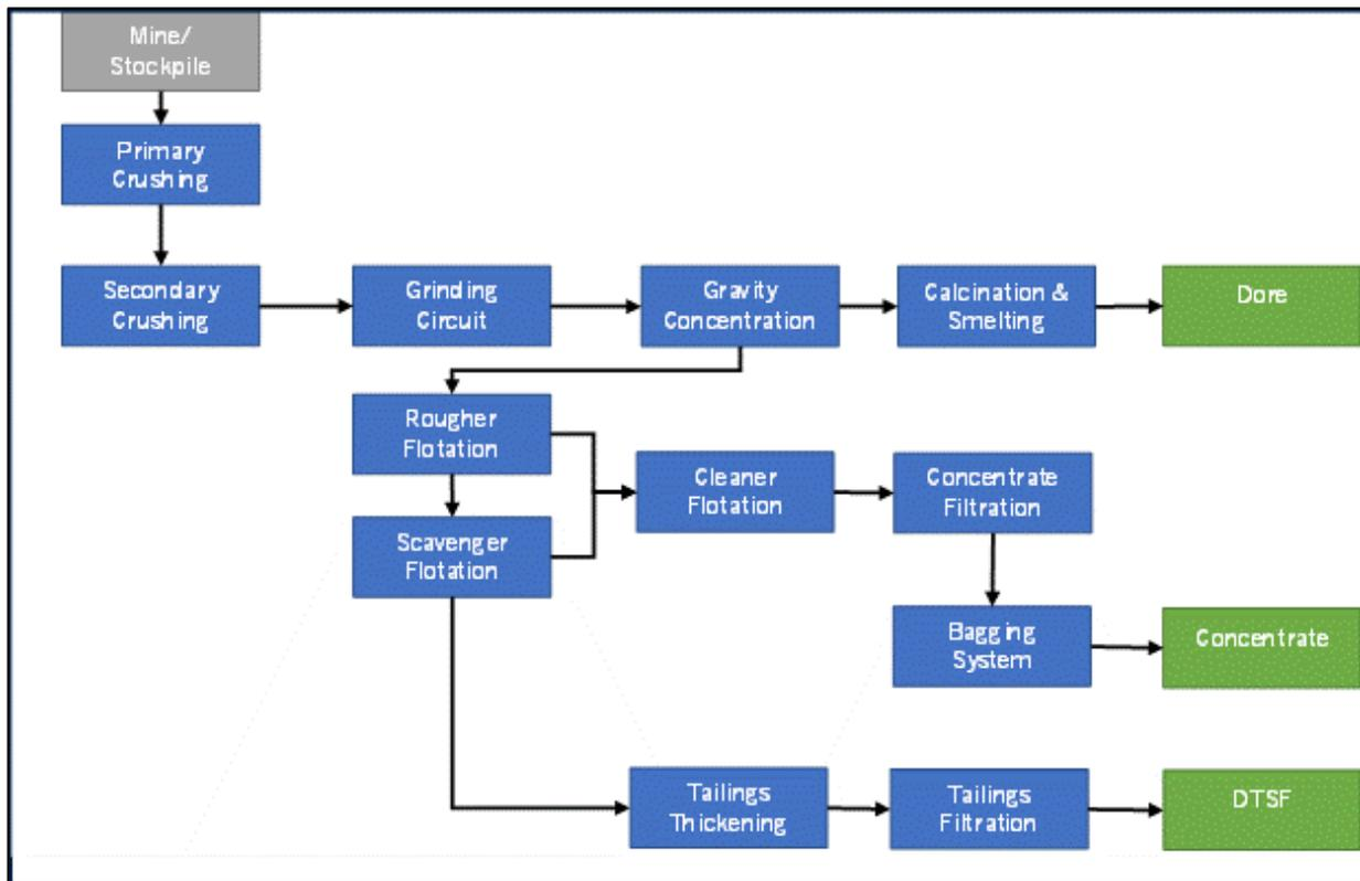
**Figure 17: Block Diagram of the Processing Flowsheet**
