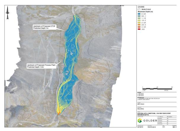
Figure 26: Maximum Flooding Depth 1-in-1000 year event (from Golder, 2022e)
