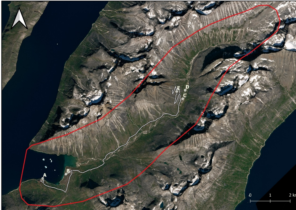
Figure 1-1: Graphic of the Overview of Project Area with major project elements, including the road between the jetty and the mine area, shown with a white line. A: Jetty, B: Camp, C: Process plant, D: Tailing storage, E: The mine.
