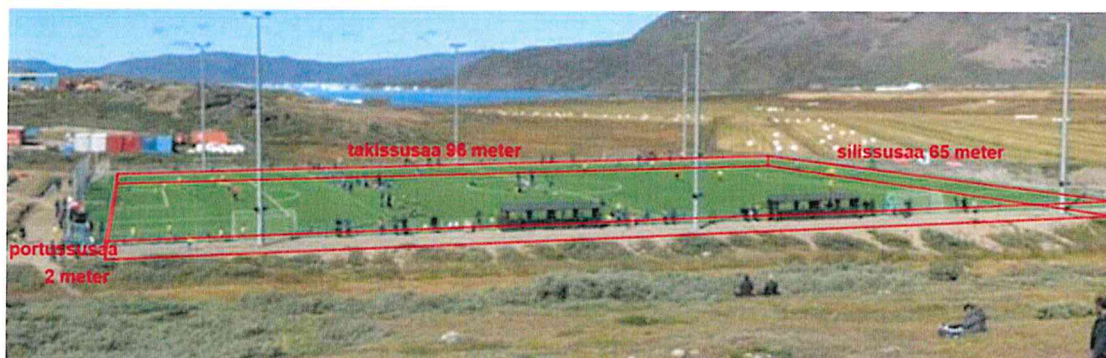
Figure 4. Each blasting operation corresponds to the size of Narsaq's football field and a depth of 2 meters. 96 x 65 x 2 meters.
