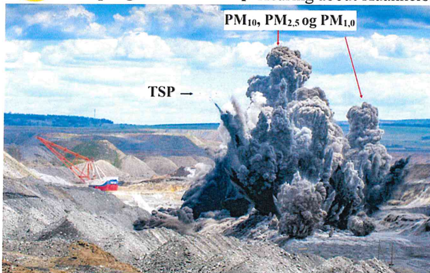
Figure 5. Open-pit blasting and dispersal of dust particles.
