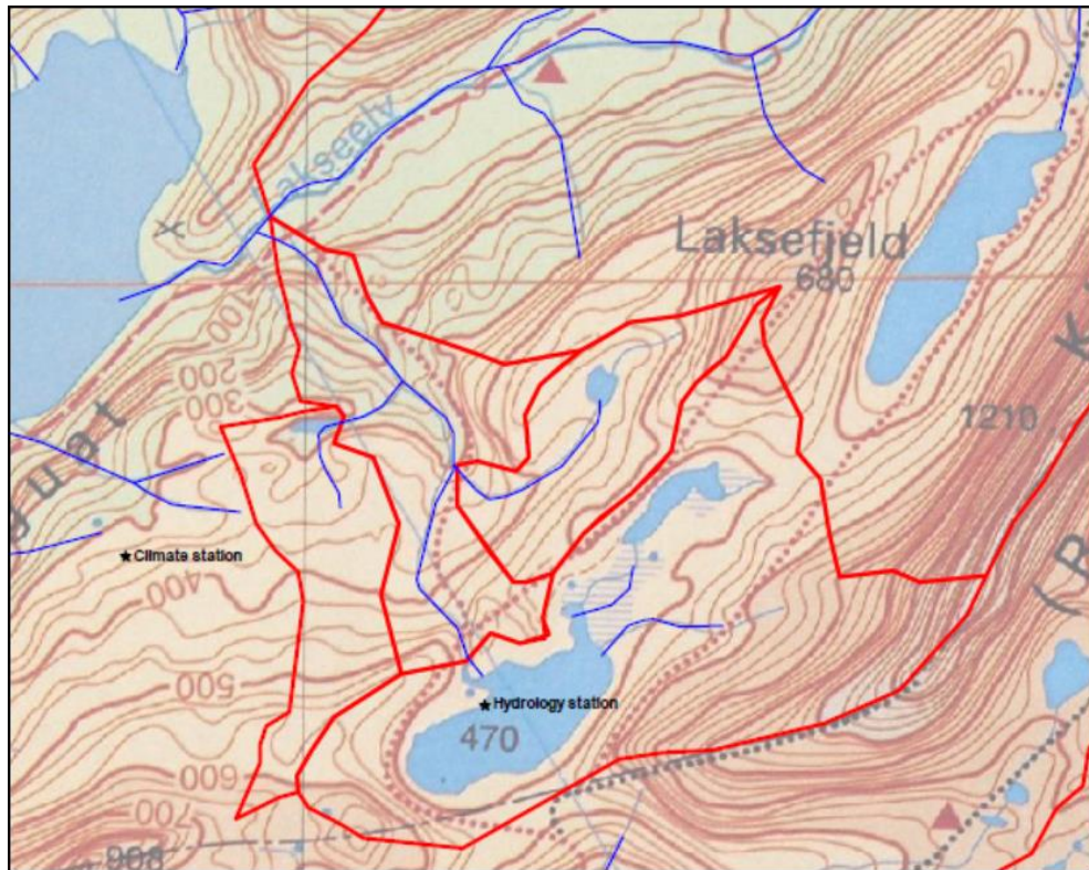
Figure 6.2 Lakseelv (top) is the main river in the area. Lake 470 is Fostersø which connects to Lakseelv via Laksetværelv. Red lines indicate the catchment areas
